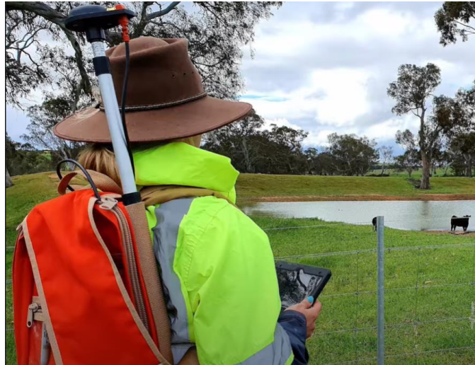
Figure 6 - SBAS receiver stored in a backpack for transport.
