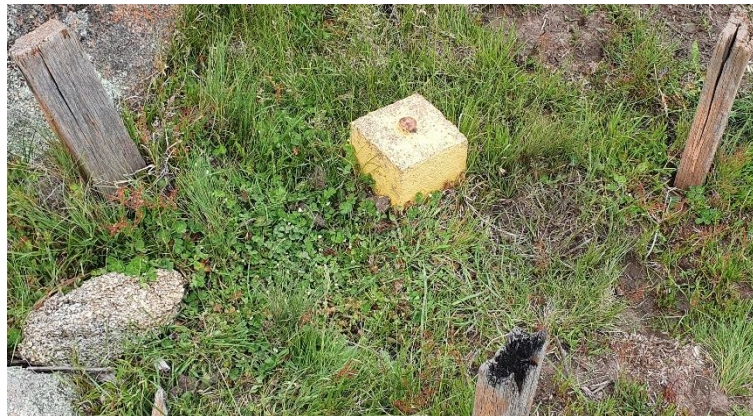
Figure 5 - Survey peg with flathead nail.
