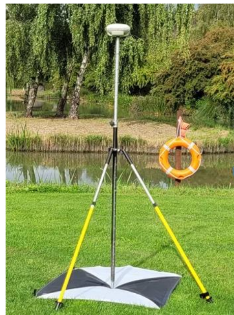
Figure 2 - UAV ground control point deployed with GNSS receiver. The GNSS receiver is recording static observations to allow high-accuracy geolocation. For satellite remote sensing such a GCP would need to be significantly larger.
